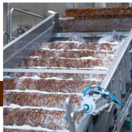
Washing lines with the automation modes enabling to decrease the water consumption at washing of the vine fruit.
